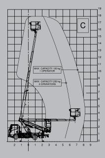
CROSSBEAMS ONE SIDE FULLY OPENED ONE SIDE CLOSED
